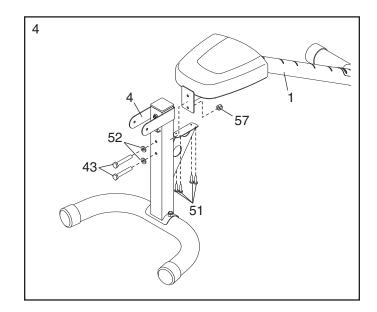
Apply a portion of the included grease to an M10 x 165mm Bolt (49). Attach the Backrest Post (15) to the Backrest Frames (16) with the Bolt, two M10 Washers (52), and an M10 Nylon Locknut (57). Do not tighten the Nylon Locknut yet.
